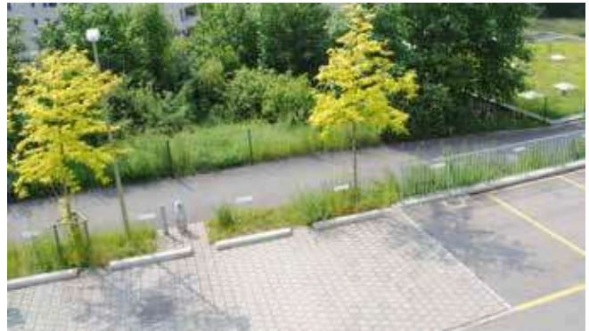
Parking lots that are adjacent to pedestrian facilities should provide a visual landscaped buffer between the parked cars and pedestrians.
